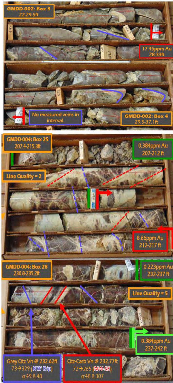
Fig. 6.10 Examples of high-grade gold intercepts from the Center Grade Zone, A) Hole GMDD-002, 8.5 – 10.1 m (28-33 ft); assay 17.45 ppm (0.51 opst) Au, B) Hole GMDD-004, 64.6-66.1 m (212-217 ft); assay 8.66 ppm (0.25 opst) Au (Burtner, 2021)
