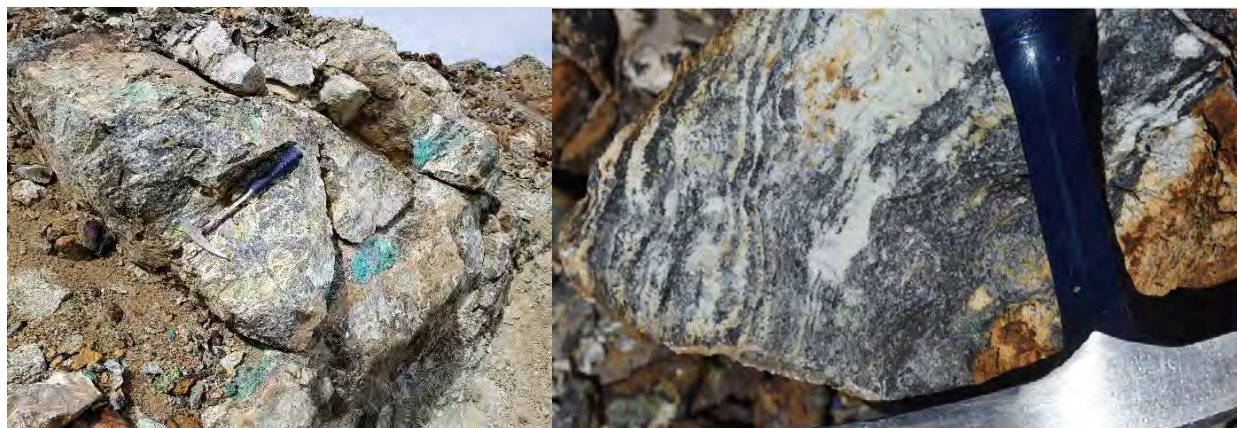
Figure 6.7 Magnetite-Copper Skarn of the Main Zone at Golden Mile. Photo on right shows metasomatic bands of mainly magnetite and calcite.
